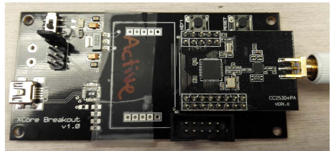
Fig. 5. Close-up of custom Texas Instruments CC2530 breakout board
